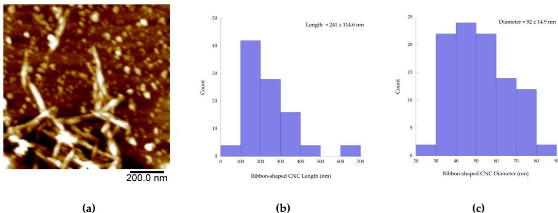
**Figure S1.** (a) AFM micrograph showing the co-existence of ribbon-shaped and spherical CNC. Histograms of (b) ribbon-shaped CNC length and (c) ribbon-shaped CNC diameter and their respective averages.
