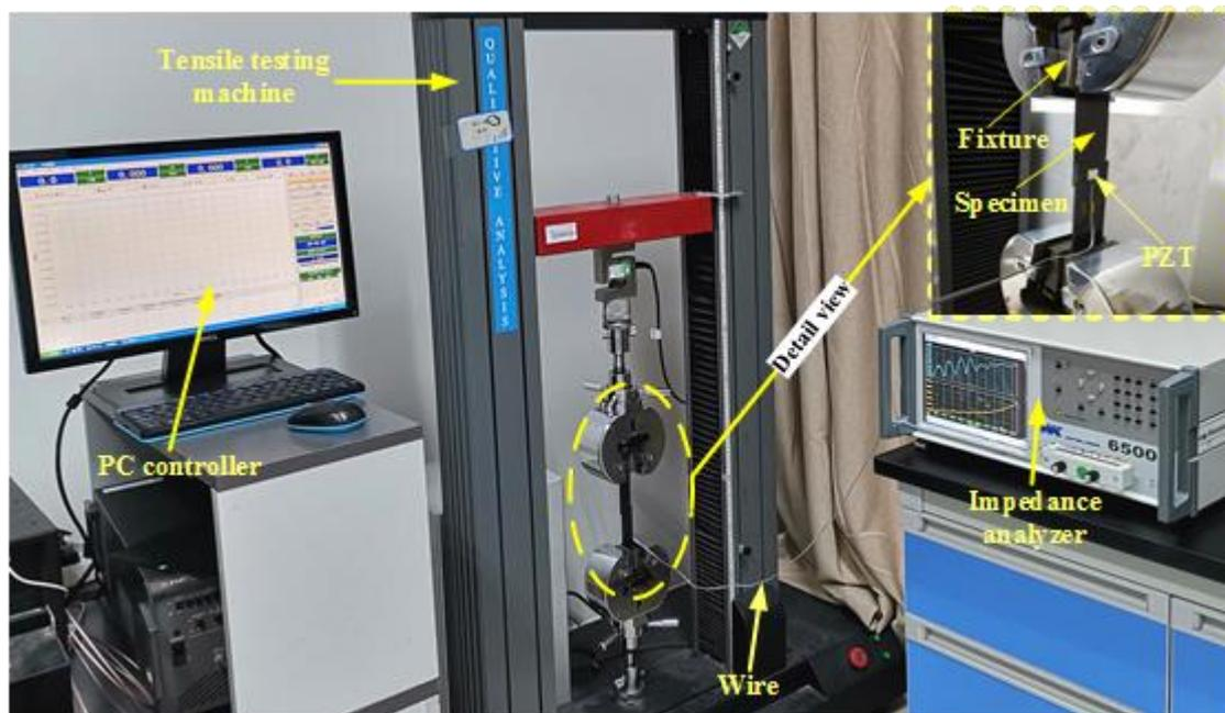
Figure 2. Testing platform for single-lap joint quasi-static behavior monitoring.
