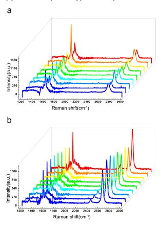
Figure 4. Raman spectra at nine random points on the surface of EG sample (a) and QFSG sample (b).
