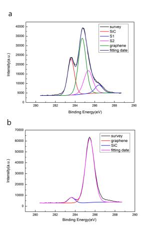
$\label{eq:Figure 3.} \textbf{X-ray photoelectric spectroscopy of EG sample (a) and QFSG sample (b)}.$
