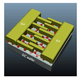
**Figure 1.** The 3D structure diagram of epitaxial graphene photodetector, the light absorption area is about 1.3 mm<sup>2</sup> while the total size of the device is about 4 mm<sup>2</sup>.
