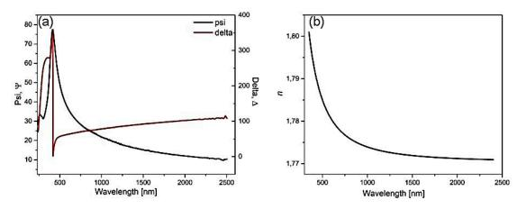
**Figure 7.** Spectral ellipsometric data ( $\Psi$ ,  $\Delta$ ) of ZnS thin film before annealing (**a**) and refractive index (*n*) extracted from the spectral dependencies of the ( $\Psi$ ,  $\Delta$ ) (**b**).
