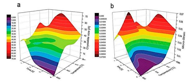
**Figure 4.** 3D graphs representing crystallite size (**a**) and micro-strain (**b**) as a function of annealing time and temperature for the studied ZnS thin films.
