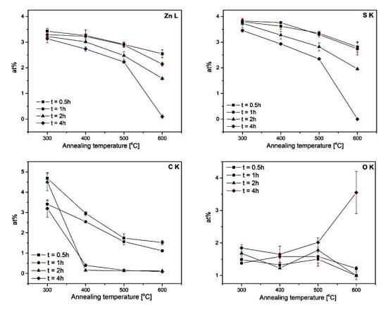
**Figure 2.** Energy-dispersive X-ray spectrometer (EDS) elemental analysis at accelerating voltage of 5 kV: the average Zn, S, C, and O concentration (at%) in the ZnS layers after annealing for 0.5, 1, 2, and 4 h as a function of annealing temperature.
