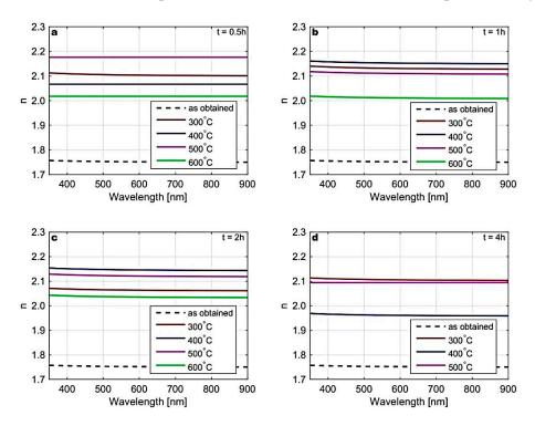
**Figure 9.** Refractive index (*n*) extracted from the spectral dependencies of the ( $\Psi$ ,  $\Delta$ ) measured for the ZnS thin films before annealing (as obtained), and annealed at 300 °C, 400 °C, 500 °C, and 600 °C for 0.5 (**a**), 1 (**b**), 2 (**c**), and 4 h (**d**).
