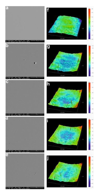
**Figure 1.** SEM images (left column) and 3D outputs obtained with Veeco/Wyko NT-1100 TM real-time optical surface profiler (right column) for ZnS film before annealing (**a**,**f**), and after annealing for 1 h at 300 °C (**b**,**g**), 400 °C (**c**,**h**), 500 °C (**d**,**i**), and 600 °C (**e**,**j**), respectively.
