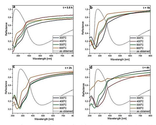
**Figure 5.** Reflectance spectra of the ZnS thin films before annealing (as obtained), and annealed at 300 °C, 400 °C, 500 °C, and 600 °C for 0.5 (**a**), 1 (**b**), 2 (**c**), and 4 h (**d**).
