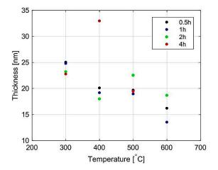
**Figure 8.** Thickness of the ZnS films as a function of annealing temperature for a given annealing time extracted from the spectral dependencies of the  $(\Psi, \Delta)$ .
