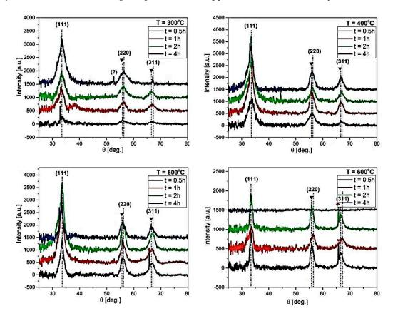
**Figure 3.** X-ray diffraction (XRD) pattern of the samples annealed at temperatures 300, 400, 500, and 600 °C for various annealing times (t) of 0.5, 1, 2, and 4 h. The red star symbol signifies the reflections originating from the Si substrate; the inverted triangles indicate the probable reflections from the twinned sphalerite.
