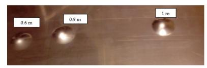
**Figure 6.** Tested metal sheet deformation after the impact of 1 kg weight from different heights: 0.6, 0.9, and 1.0 m.
