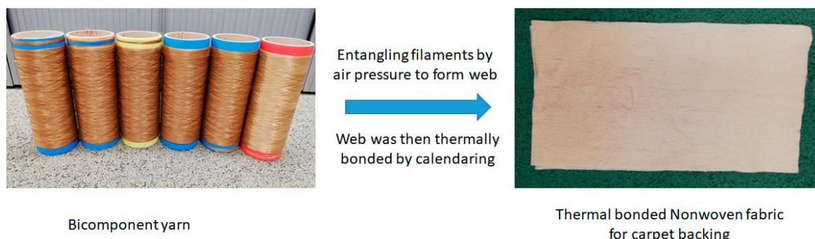
**Figure 2.** Bicomponent filaments and thermal bonded nonwoven fabric.
