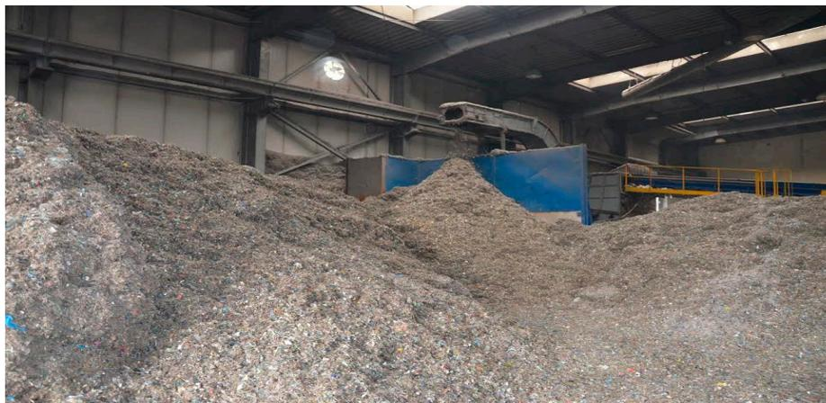
**Figure 1.** Alternative fuel storage method in the production and storage hall (own photo).
