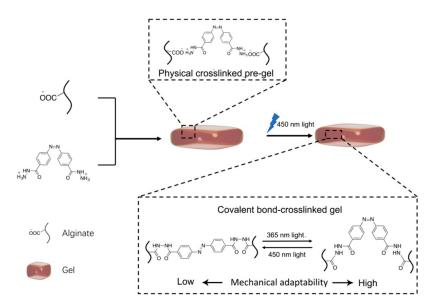
Figure 1. The scheme of the fabrication of Azo-alginate gel.
