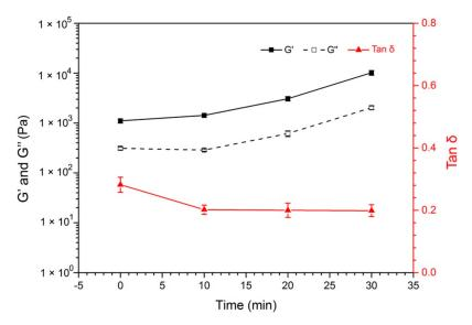
Figure 5. The effect of 365 nm light irradiation time on Azo-alginate gel mechanical properties.
