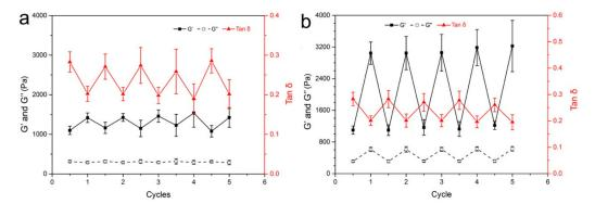
**Figure 6.** The reversible gel mechanical adjustment induced by (**a**) 10 min and (**b**) 20 min of 365 nm light and 450 nm light irradiation.
