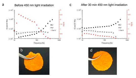
**Figure 3.** The change in rheological properties of (**a**) the pre-gel of Azo-alginate to the shearing frequency, and (**b**) its image. (**c**) The change in rheological properties of Azo-alginate gel to the shearing frequency, and (**d**) its image.
