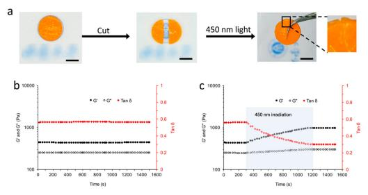
**Figure 7.** (a) The 450 nm light induced gel splicing. In addition, the mechanical properties of the gel stack (b) without and (c) with 450 nm irradiation.
