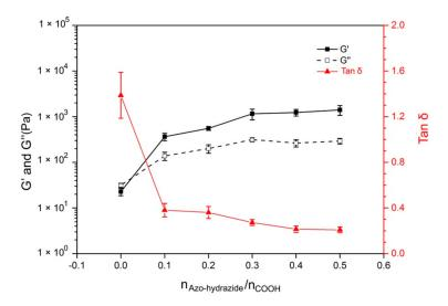
**Figure 4.** The effect of the molar ratio of linker and alginate carboxyl groups on gel mechanical properties, where  $n_{Azo-hydrozide}$  is the molar quantity of the added Azo-hydroazide, and  $n_{COOH}$  is the total carboxyl group molar quantity in the gel. All samples were analyzed by a time-scan rheological test with a fixed frequency and strain of 50 Hz and 5% respectively.
