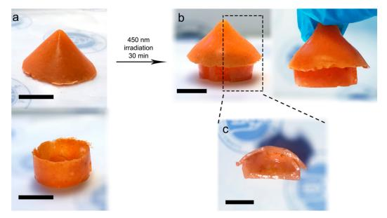
**Figure 8.** (a) Chemically crosslinked gel parts. (b) The gel structure spliced from gel parts by the 450 nm light irradiation. (c) Longitudinal cut surface of the gel structure, with hollow cavity. (Scale bar = 1 cm).
