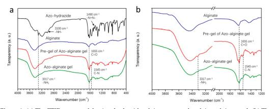
**Figure 2.** (a) The FTIR spectra of the Azo-hydrazide, alginate, pre-gel and Azo-alginate gel. (b) The FTIR spectra of the alginate pre-gel and Azo-alginate gel, showing the spectra at wavenumber ranges of  $4000-3000 \text{ cm}^{-1}$  and  $2500-1200 \text{ cm}^{-1}$ .
