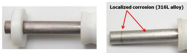
**Figure 4.** Sample used for the crevice corrosion tests.
