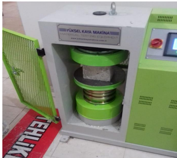
Figure 10. Appearance of samples in compressive strength tester.
