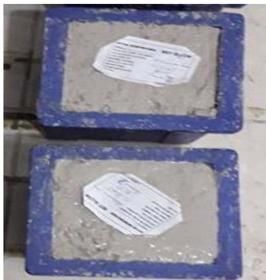
Figure 6. Pumice binder mortar for optimum binder fixation.
