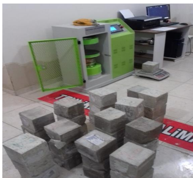
Figure 9. Samples prepared for compressive strength tests.
