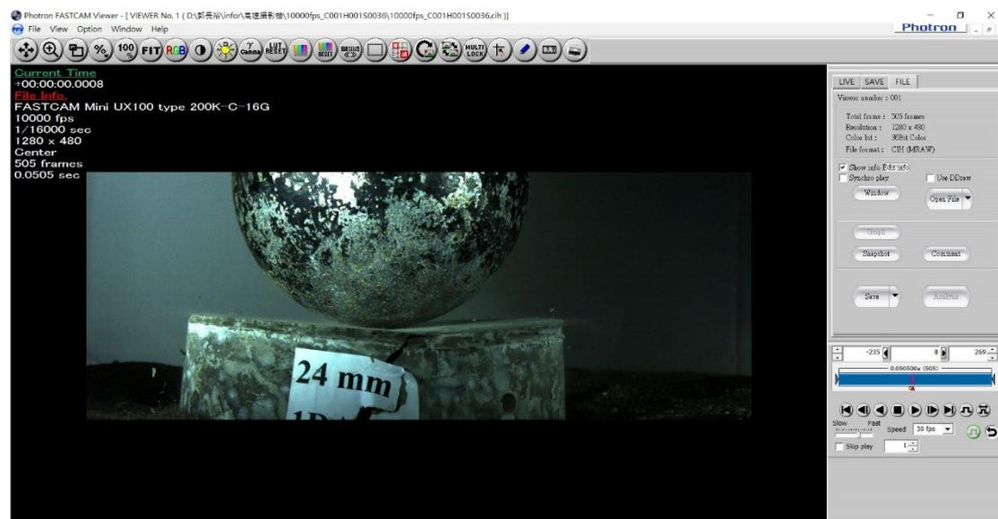
Figure 12. The image of benchmark specimen after the steel ball impact taken by high speed camera.
