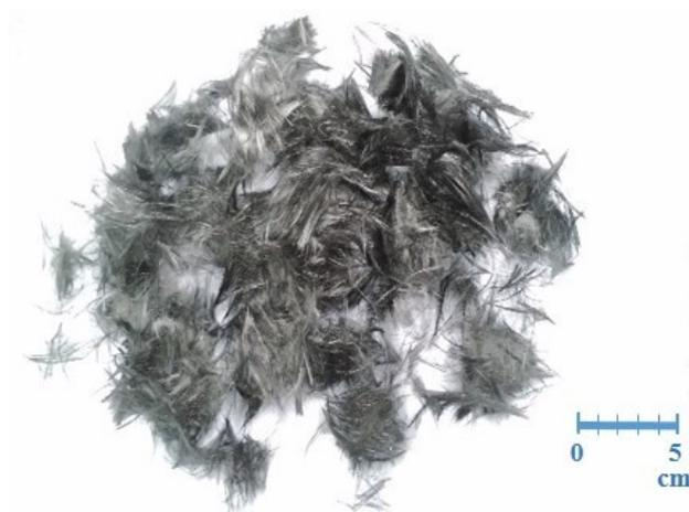
**Figure 9.** Appearance of carbon fibers after dispersion.
