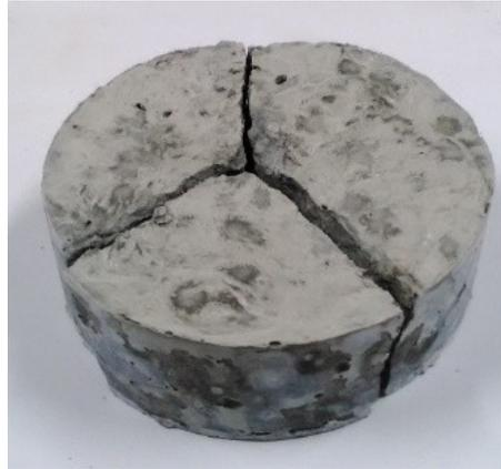
**Figure 14.** The fracture photo of the most specimen after impact test.
