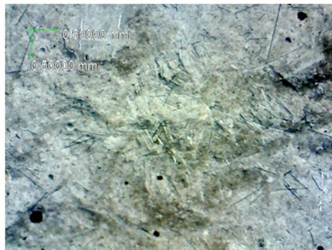
**Figure 15.** The optical microscopic photo of the specimen unprocessed carbon fibers after impact test.
