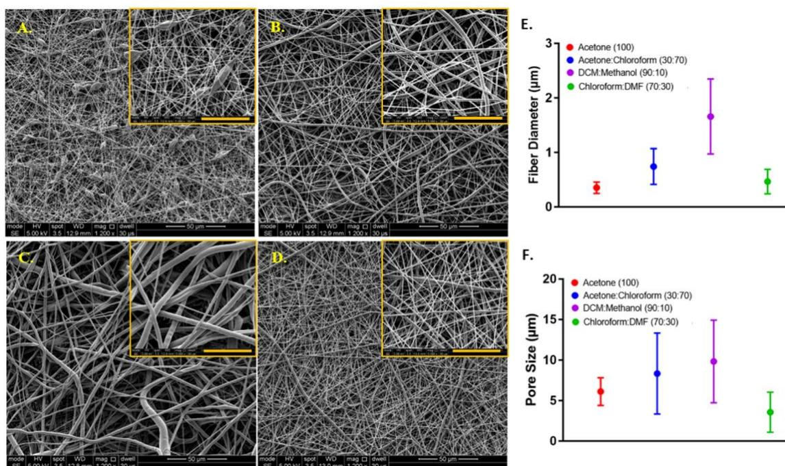
**Figure 6.** Morphological characterisation of the electrospun PCL fibres, where polymer solutions were prepared with different solvents. SEM image of PCL electrospun prepared by dissolving PCL in (A) acetone (100), (B) acetone:chloroform (30:70), (C) dichloromethane (DCM):methanol (90:10), (D) chloroform:dimethylformamide (DMF) (70:30). The graphs show (E) the fibre diameter and (F) the pore size distributions, respectively. Yellow scale bars represent 20 μm.
