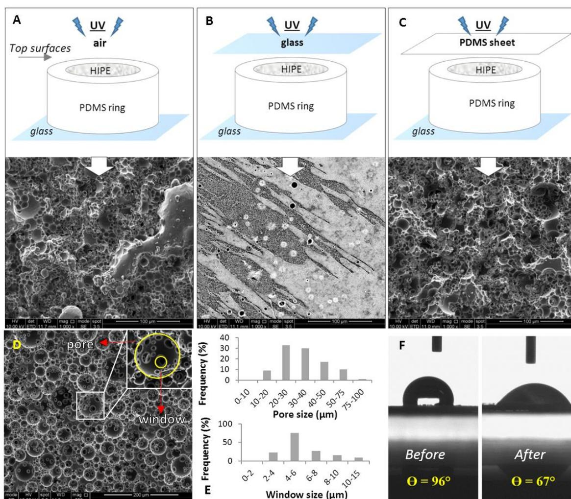
**Figure 2.** Scanning electron microscope (SEM) images of the top surfaces PCL polyHIPEs cured in contact with; (A) air, (B) glass, and (C) polydimethylsiloxane (PDMS) sheet. (D) SEM image of the transverse section of PCL polyHIPEs. (E) Pore size and window size distributions of the inner section. (F) Contact angle measurements of a water droplet on PCL polyHIPE before and after air plasma treatment ( $n = 3$ ).
