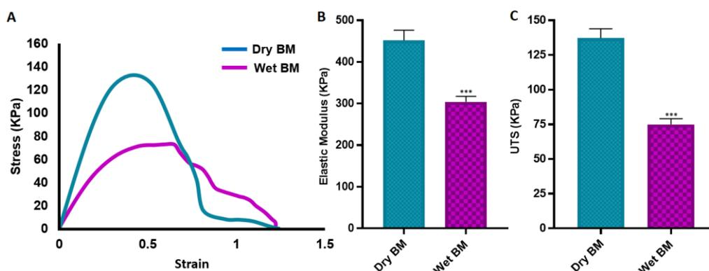
**Figure 8.** Mechanical properties of the BM under dry and wet conditions. (A) Representative stress-strain curves, (B) elastic modulus, (C) ultimate tensile strength (UTS) of the BMs under dry and wet conditions (\*\*\*)  $p \leq 0.001$ ,  $n = 3$ ).
