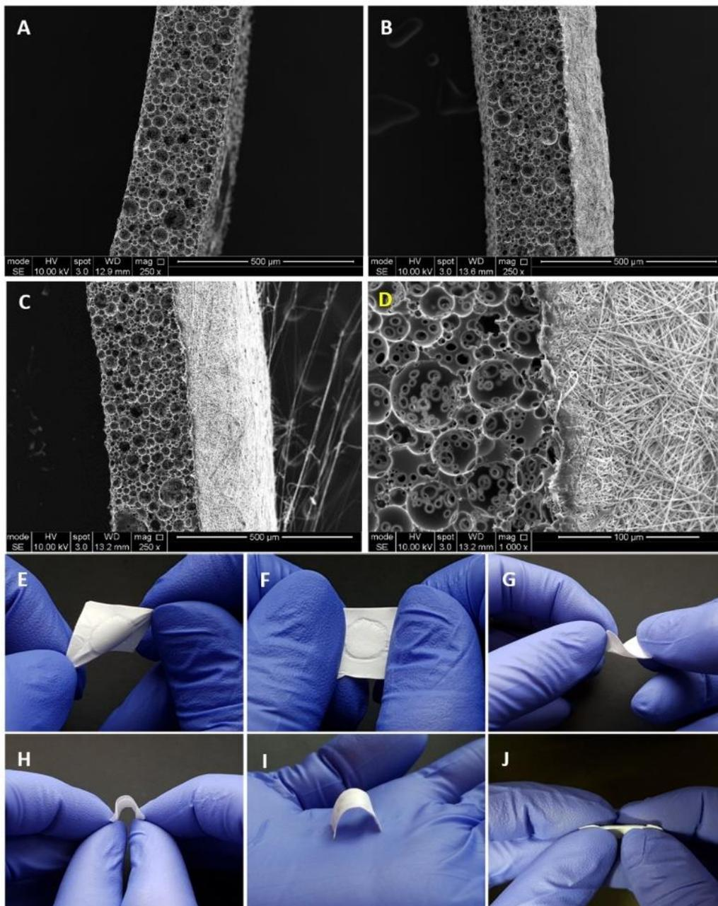
**Figure 7.** SEM images of (A) 250 μm sectioned PCL polyHIPE layer, (B) 20 min PCL electrospun on PCL polyHIPE, (C) 40 min PCL electrospun on PCL polyHIPE, (D) Higher magnification SEM image showing the border of two layers. Macro images of the bilayer PCL barrier membrane (BM) to show the suitability of the design for (E–F) stretching in different axes, (G–H) bending, (I) space making, and (J) side view of the BM to show the integration of the two layers.
