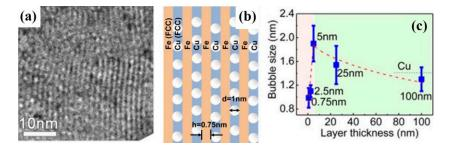
**Figure 17.** (a) TEM images of irradiated fully coherent 0.75 nm Cu/Fe multilayer. (b) Schematics illustrate that in a coherent 0.75 nm Cu/Fe multilayer, He bubbles prefer to nucleate in Cu layers and are constricted to reside inside Cu layers. (c) The variation of He bubble density with layer thickness h [20].
