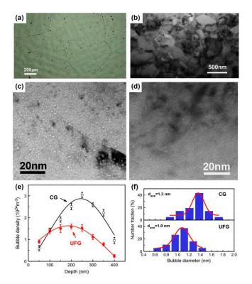
**Figure 9.** (**a**) An optical microscopy image of as-received coarse-grained (CG) Fe–Cr–Ni alloy. (**b**) TEM micrograph of ultrafine grain (UFG) Fe–Cr–Ni alloy after equal channel angular pressing (ECAP). (**c**,**d**) Under focused TEM micrograph of He ion irradiated CG and UFG Fe–Cr–Ni alloys. (**e**) Depth dependent bubble density in irradiated CG and UFG Fe–Cr–Ni alloy. (**f**) Bubble diameter distribution in the peak damage region of He ion irradiated CG and UFG Fe–Cr–Ni alloys [37].
