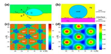
**Figure 7.** (a) Schematic of wetting model on interfaces. (b) Schematic of a void wetting a single misfit dislocation interaction (MDI) where W > 0 at a Cu/Ag interface. (c) Misfit dislocation network in the cube-on-cube Cu/Ag interface. Atoms shown are on the Cu side of the interface and colored by coordination number. (d) Contour plot of the location-dependent interface energy of a Cu/Ag interface. Black contours correspond to zero wetting energy [33].
