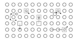
**Figure 1.** Schematic illustration of defect configurations and jump processes relevant for He diffusion without and with irradiation [8].
