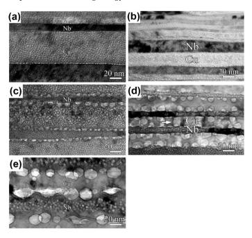
**Figure 8.** TEM images of accumulative roll bonding (ARB) Cu/Nb after He ion irradiation with different layer thickness, implantation dose and temperature. (**a**) 58 nm,  $2 \times 10^{17}$  ions/cm<sup>2</sup>, room temperature (RT); (**b**) 16 nm,  $2 \times 10^{17}$  ions/cm<sup>2</sup>, RT; (**c**) 58 nm,  $6.5 \times 10^{17}$  ions/cm<sup>2</sup>, RT; (**d**) 16 nm,  $2 \times 10^{17}$  ions/cm<sup>2</sup>, 450 °C [22].
