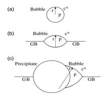
**Figure 2.** Illustration of interfacial effects on bubble nucleation at high temperatures; (**a**) spherical nucleus in the matrix, (**b**) lenticular nucleus at a grain boundary (GB), (**c**) truncated lenticular nucleus at a GB-precipitate, all assumed to have the same volume [8].
