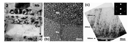
**Figure 12.** (a) Low magnification TEM micrograph of 100 nm Cu/Nb multilayer irradiated with He ions at 150 keV with a dose of  $1 \times 10^{17}$  ions/cm<sup>2</sup>. (b) Defocused HRTEM micrograph of Cu/Nb interfaces indicated cavities in each constituent has 1 nm in diameter and aligned along the interface. (c) 2.5 nm Cu/Nb multilayers subjected to He ion irradiation at 150 keV with a dose of  $1 \times 10^{17}$  ions/cm<sup>2</sup> [7].
