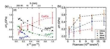
**Figure 18.** (a) Irradiation hardening in He ions irradiated Ag/V, Ag/Ni, Cu/V multilayers scaling with layer thickness. (b) Fluence dependence of irradiation hardening in He ion irradiated Cu/V multilayers [39].
