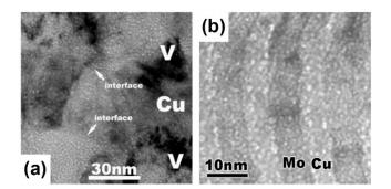
**Figure 11.** Under focused TEM images of He ion irradiation on multilayers with a dose of  $6 \times 10^{16}$  ions/cm<sup>2</sup>. (a) Cu/V multilayers [19]; (b) Cu/Mo multilayers [40].
