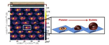
**Figure 4.** Left: Location-dependent energy of Cu/Nb interfaces. The bright, high-energy regions are heliophilic. Right: A He platelet transforms into a bubble once it has grown to occupy the entire heliophilic patch on which it nucleated [28].
