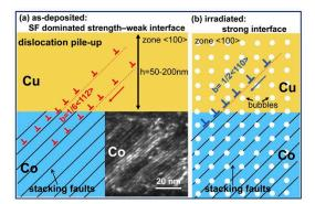
**Figure 21.** Hypothetical schematics illustrate different strengthening mechanisms in as-deposited and irradiated Cu/Co (100) multilayers at large h (h = 50-200 nm). (**a**) In the as-deposited state, partial dislocations can transmit across the Cu/Co interface relatively easily; (**b**) After radiation, high-density He bubbles are distributed both along the layer interface and within the layers [56].
