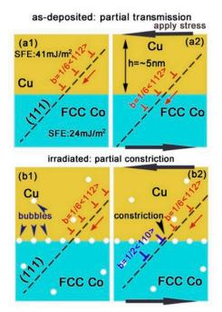
**Figure 20.** Hypothetical schematics compare strengthening mechanisms in as-deposited and irradiated Cu/Co (100) multilayers at small h (h = 5 nm). (**a1**, **a2**) In as-deposited films, partials can trespass layer interfaces owing to the low stacking fault energy of Cu and Co. (**b1**, **b2**) However, after radiation, bubbles at the layer interface disrupt the transmission of partials [56].
