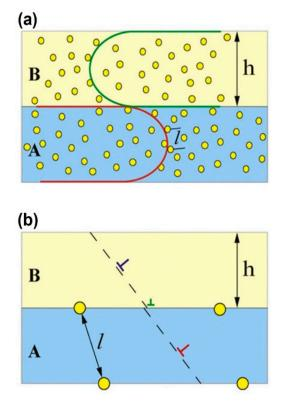
**Figure 19.** Schematic illustration of the bubble distribution in multilayers (the circles indicate bubbles). (a) When the layer thickness is a few tens of nanometers, h > l and the deformation is via confined layer slip. (b) When the layer thickness is of the order of a few nanometers, h < l, the yield strength is determined by the crossing of single dislocations across interfaces [43].
