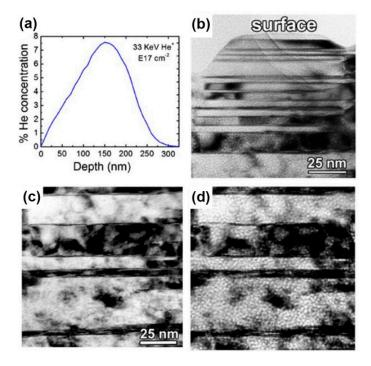
**Figure 15.** (a) Depth profile of He concentration in nanotwined (NT) Cu film implanted to a dose of  $1 \times 10^{17}$  ions/cm<sup>2</sup> with 33 keV He ions, calculated using the stopping and range of ions in matter (SRIM). (b) Under-focused (-2 um) bright field TEM image from near surface. (c,d) Near-focus and under-focused (-2 um) bright field TEM images from a depth of 150 nm (peak He concentration) [50].
