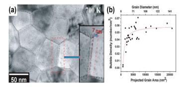
**Figure 10.** (a) Over-focused bright field TEM images of 10 keV He ion irradiation on nanocrystalline iron at calibrated temperatures of 700 K. (b) Areal bubble density (number/nm<sup>2</sup>) vs. grain size (area) for 10 keV He ion irradiation on nanocrystalline iron at 700 K [38].
