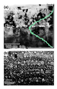
**Figure 13.** (a) Cavities in irradiated Cu/Nb multilayers with 120 nm layer thickness. (b) Cavities in He ion irradiated Cu/Nb multilayers with 5 nm layer thickness [46].
