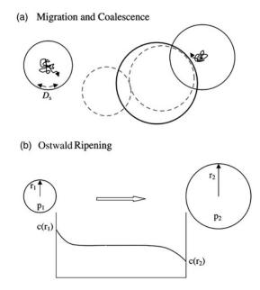
**Figure 3.** Schematic illustration of the two main bubble coarsening mechanisms, (**a**) migration and coalescence via surface diffusion, (**b**) Ostwald ripening due to He fluxes driven by differences in the thermal equilibrium He concentrations in the vicinity of small and large bubbles [8].
