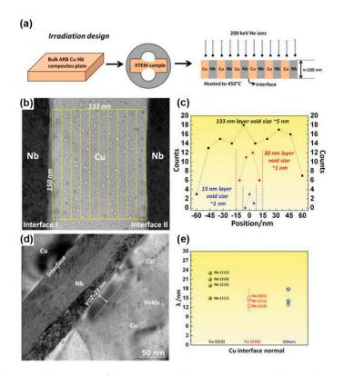
**Figure 5.** (a) Schematic illustration of the He ion irradiation experimental procedures. (b) Illustration of the method to determine the void number density in Cu layers. (c) Plot of the number density of voids as a function of distance from the center of the layer in 133 nm-, 30 nm- and 15 nm-thick Cu layers. (d) Under-focus TEM image showing a void-denuded zone (VDZ) near a Cu/Nb interface. (e) Widths of VDZs near Cu/Nb interfaces sorted by their plane orientations [31].
