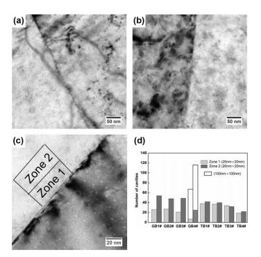
**Figure 16.** (**a**,**b**) Cavities near general a grain boundary and twin boundary in Cu after He ion irradiation. (**c**) high-magnification micrograph of the cavities near the twin boundary. (**d**) Statistical data of the cavities number adjacent to two types of the boundaries [51].
