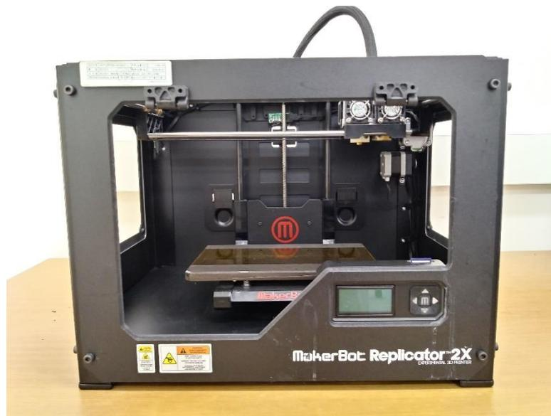
**Figure 3.** Fused deposition modelling (FDM) 3D printer.
