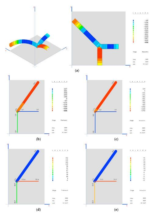
**Figure 19.** (a) The stability of the structure is guaranteed between 45 kN and the 624 kN because in that range the arches work in compression completely; (b) construction phase of prestressing; (c) final construction phase; (d) elastic limit in the prestressing phase of construction; (e) elastic limit in final construction phase.
