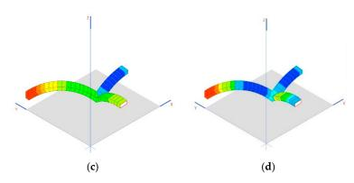
**Figure 9.** (**a**,**c**) Tractions in the dome with connecting rods at 45°; (**b**,**d**) traction in the dome with connecting rods at 60°.
