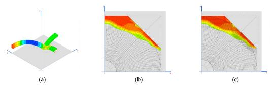
Figure 10. (a) Stresses in the arches; (b) traction stresses MPa; (c) plasticized areas (shaded area).
