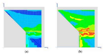
**Figure 17.** (**a**) The tension in the vaults are of the order of 2 MPa, considering the same conditions as for the dome; (**b**) the possibility of cracks in the direction of the gallery for tensioners greater than 0.3 MPa.
