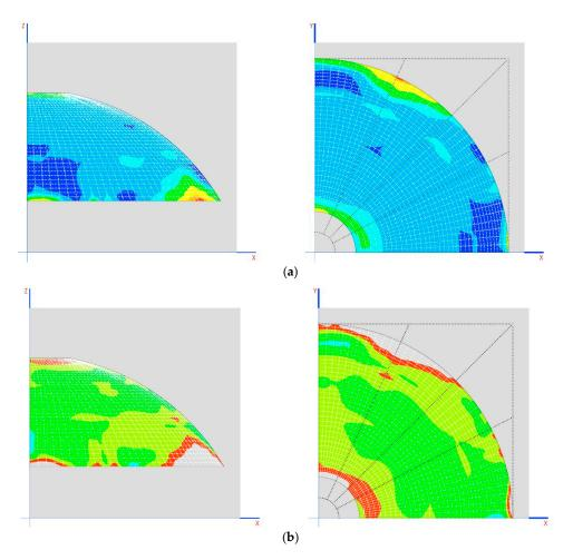
Figure 15. (a) Possible appearance of cracks without affecting the stability of the structure; (b) transparent areas are the most stressed.
