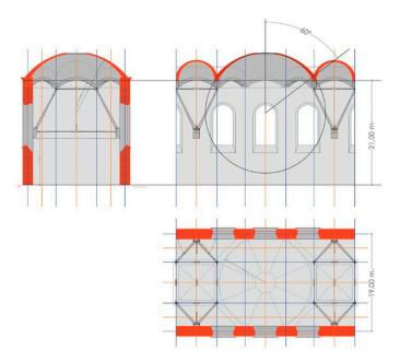
Figure 2. Geometric scheme used for the calculation from the original image.
