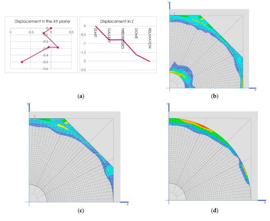
**Figure 13.** (a) Diagram of the displacement of the connecting rod support (mm); (b) traction in the dome (MPa) in the penultimate phase of construction; (c) tractions in the dome (MPa) in the last phase of construction; (d) behavior of the dome without the tympanums working.
