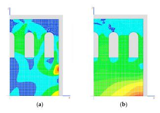
**Figure 18.** (**a**) Tension in the wall only to compression; (**b**) no noticeable traction stresses at any point on the wall.
