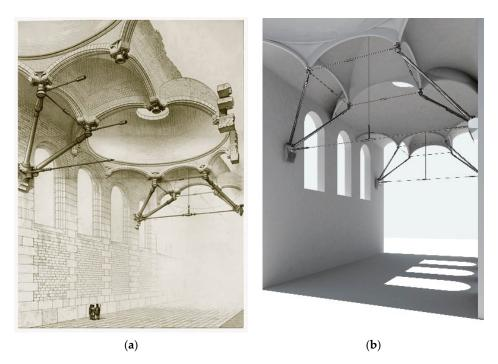
**Figure 1.** (a) Project proposed by Viollet-le-Duc for an ideal structure. (From *Entretiens sur l'architecture,* published in 1868). (b) Three-dimensional image recreated with AutoCAD + 3D Studio + Maya.
