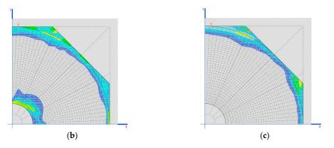
**Figure 12.** (a) Scheme of displacement of the point of anchorage of the connecting rod with the arches; (b) traction in the dome (MPa) in the penultimate phase of construction; (c) traction in the dome (MPa) in the last phase of construction.
