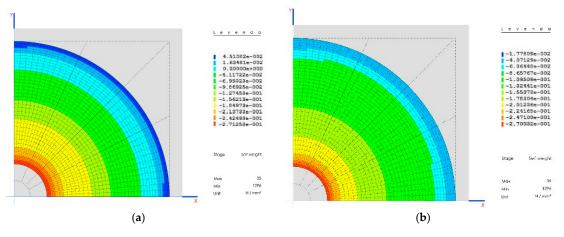
Figure 6. (a) Parallel stress; (b) the whole dome working in compression.
