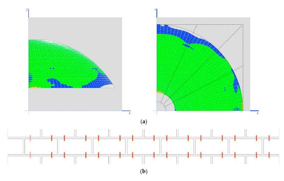
**Figure 16.** (a) Main tension is in the direction of the horizontal plane; (b) increased tensile strength with metal connectors placed as shown.
