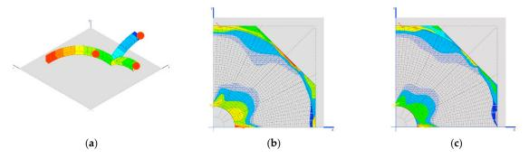
**Figure 8.** (a) Situation of the worst sections for the axial stress of the structural stone arches; (b) location of traction in the dome for the 120 mm crosspiece, up to 0.852 MPa; (c) location of traction in the dome for the 40 mm crosspiece, up to 0.856 MPa.
