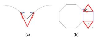
**Figure 5.** (a) Diagram in section view of the operation of the vault thrust; (b) diagram in plan view of the operation of the vault thrust.
