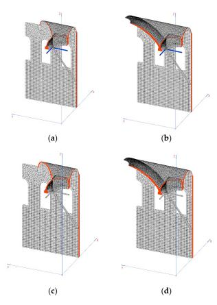
**Figure 11.** Diagrams of the different phases of construction: (a) gallery, (b) tension, (c) dome, and (d) relaxation.
