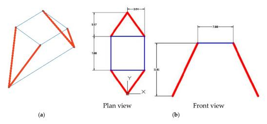
**Figure 3.** (**a**) Three-dimensional geometric diagram of the connecting rods and crosspieces; (**b**) geometric diagram of the system of connecting rods and crosspieces working together.
