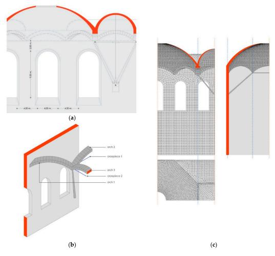
**Figure 7.** (a) Diagram of the proportions and measurements for the development of the threedimensional model; (b) name of the structural elements for the model and for this study; (c) diagram of the connecting rod–arch support.
