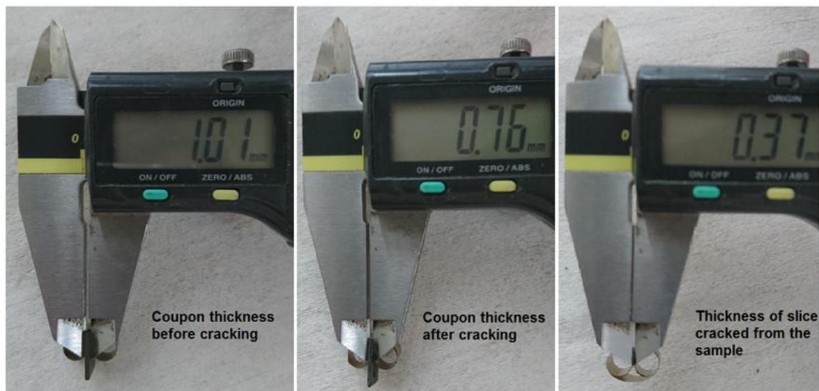
**Figure S5.** Thickness values of the Ti-base alloy before cracking (left), after cracking (middle) and of a broken slice (right), pretreated at 1173 K.
