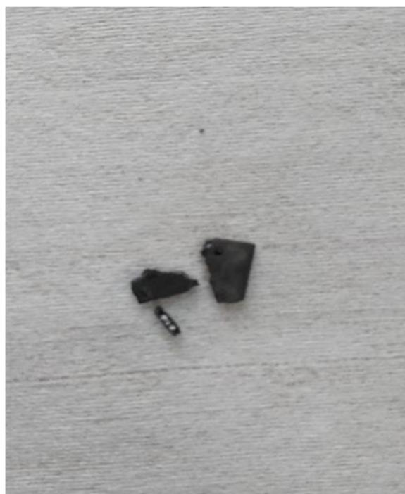
**Figure S6.** Broken Ti-base alloy coupon after cracking pretreated at 1273 K.
