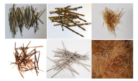
Figure 1. Samples of steel and copper fibres (top row), and basalt, plastic, and coconut fibres (bottom row).
