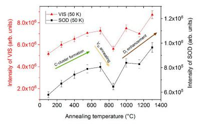
**Figure 4.** Integrated intensities of the VIS regime (1.5–2.15 eV) and SOD regime (0.73–1.08 eV) as a function of annealing temperature. Mechanisms explaining the curve characteristics are indicated in the diagram. The spectra were acquired with the 405 nm laser and the InGaAs detector at a measuring temperature of 50 K.
