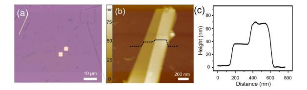
**Figure S1.** (**a**) OM and (**b**) AFM image of exfoliated TaSe3 flakes on 300 nm SiO<sub>2</sub>/Si substrate. (**c**) Line profile of the corresponding TaSe<sub>3</sub> flake, as marked in (**b**).
