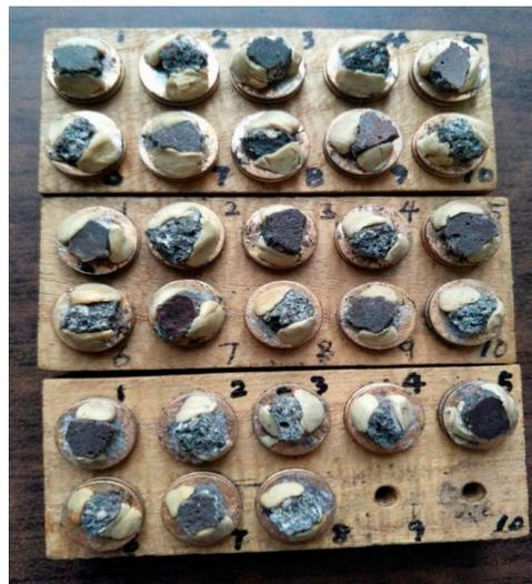
**Figure 4.** Crushed specimens immersed for 0 d, 30 d, and 50 d polymer concrete (PC).
