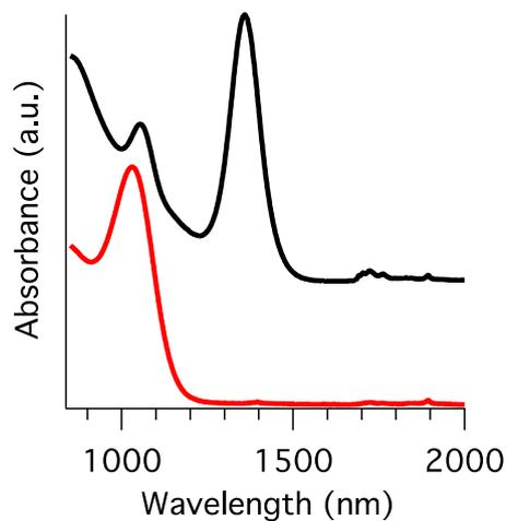
**Figure S2.** Optical absorbance spectra of PbSe nanocrystals after washing. Bottom curve has an excitonic peak at 1032 nm corresponding to a diameter of ~3 nm, top curve has an excitonic peak at 1360 nm have a diameter of ~4 nm.
