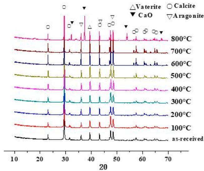
Figure 3. XRD patterns of shell powder calcined at different temperatures.
