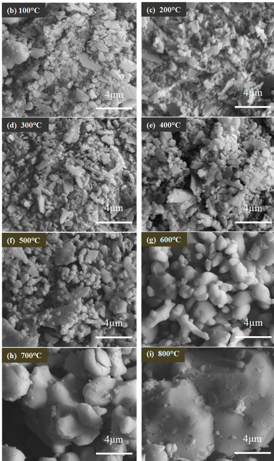
Figure 5. Micrographs of shell powders calcined at different temperatures.
