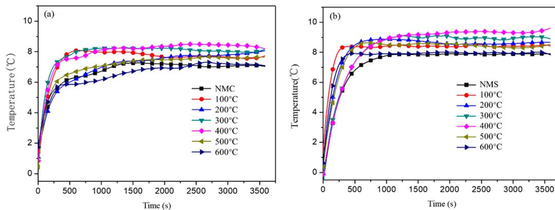
**Figure 7.** The temperature difference between inside and outside of plates coated with calcined shell powder as fillers (a) cement board, (b) steel plate. NMC and NMS represent cement board and steel plate coated with the coating filled by the as-received shell powder.
