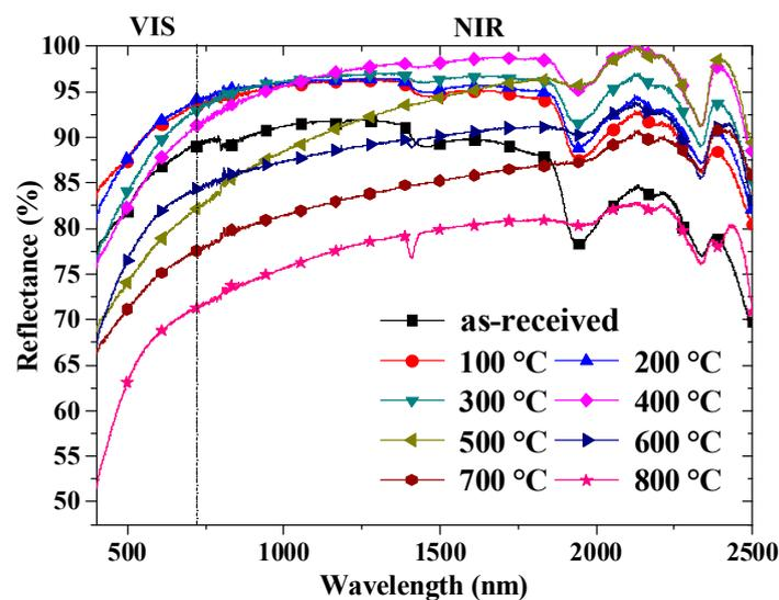
Figure 6. The reflectance of the shell powder calcined at different temperatures.
