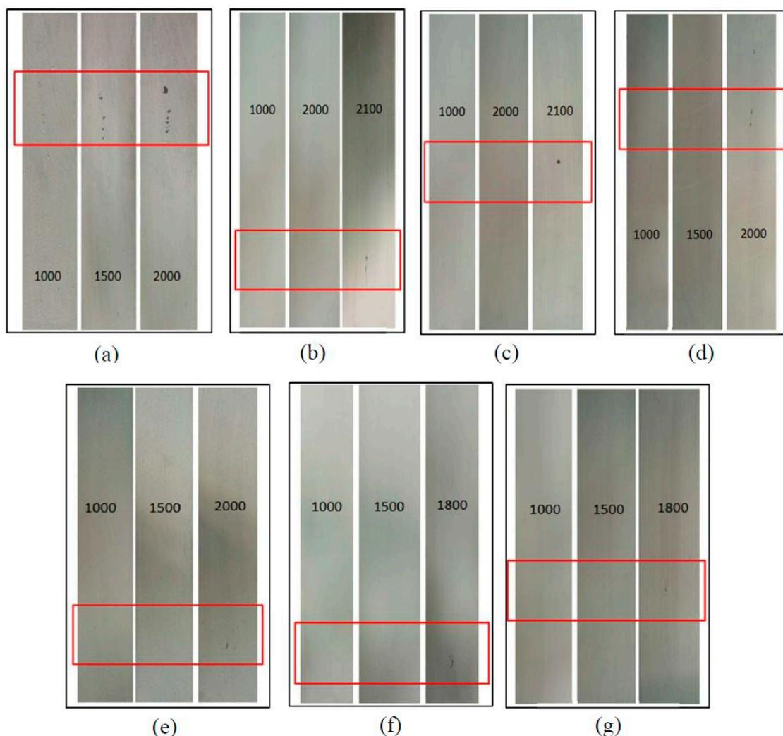
**Figure 9.** The scrub resistance of coatings with shell powder calcined at different temperature. (a) as-received; (b) 100 °C; (c) 200 °C; (d) 300 °C; (e) 400 °C; (f) 500 °C; (g) 600 °C.
