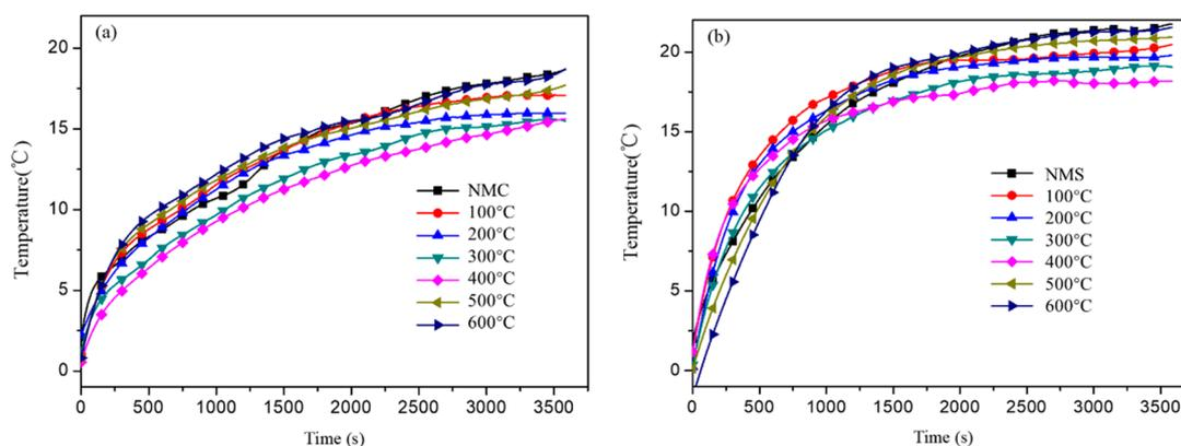
**Figure 8.** The external temperature rise of coatings with calcined shell powder (a) cement board, (b) steel plate. NMC and NMS represent coating with as-received shell powder.
