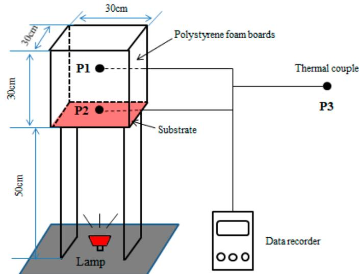
**Figure 2.** Schematic diagram for testing the heat insulating properties of coatings.
