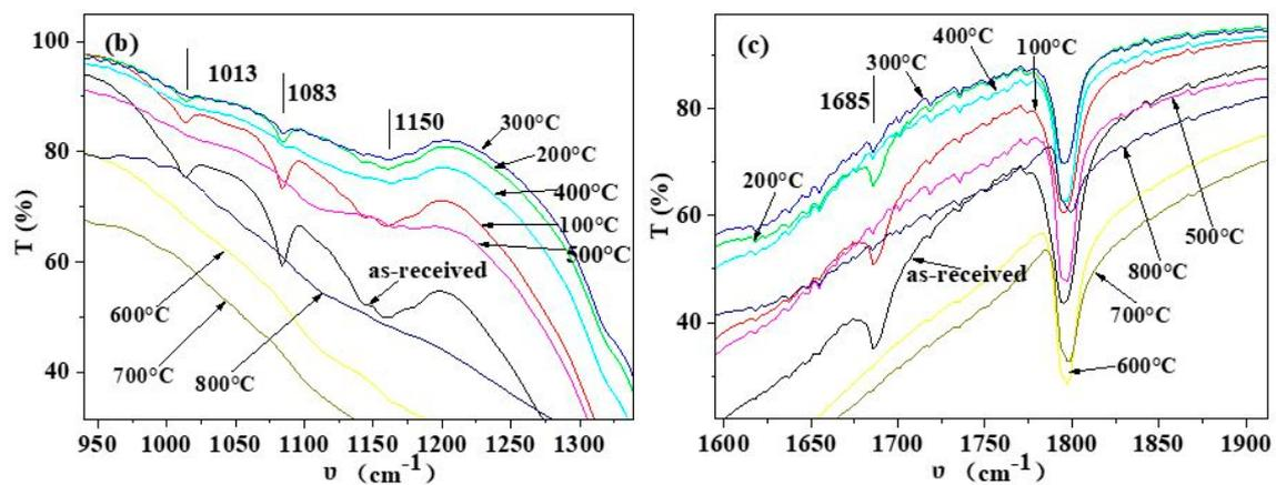
**Figure 4.** FT-IR spectra of shell powder calcined at different temperatures. (a) Full image, (b) enlarged the image of zone R1, (c) enlarged image of zone R2.
