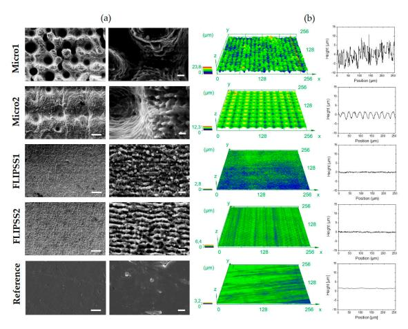
**Figure 1.** Surface characterization of laser-structured Ti6Al4V specimens. (a) Scanning electron microscope images (StereoScan360), scale bars left:  $10 \mu m$ , right:  $1 \mu m$  and (b) confocal laser scanning microscope images (LEXT OLS 4000), square side length:  $256 \mu m$ , with corresponding elevation profile of laser irradiated structures and polished Ti6Al4V reference.
