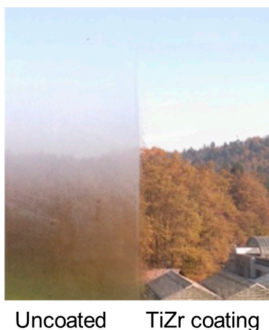
Figure 6. The anti-fogging effect of the TiZr coating on the office window. The picture was taken on 20 October 2017 after one month of exposure time.
