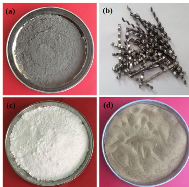
**Figure 1.** Raw materials used in study: (a) Class I fly ash, (b) Milling steel fiber, (c) Nano-SiO<sub>2</sub>, and (d) water reducing agent.
