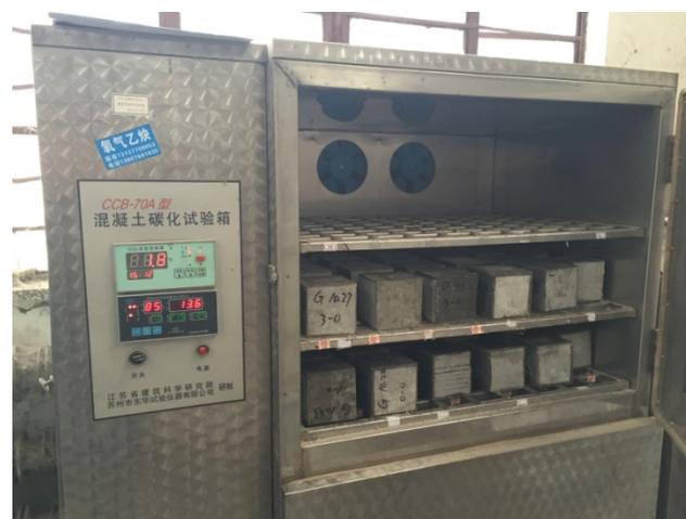
Figure 2. Carbonation test setup.
