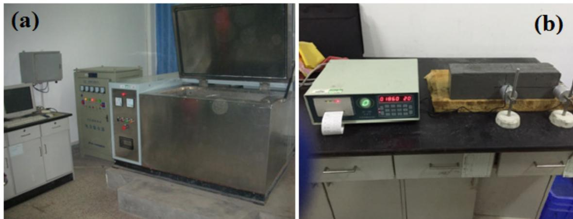
**Figure 4.** Freeze-thaw cycle test setup: (a) Freeze-thaw cycle test machine, (b) Measurement of dynamic modulus of elasticity.
