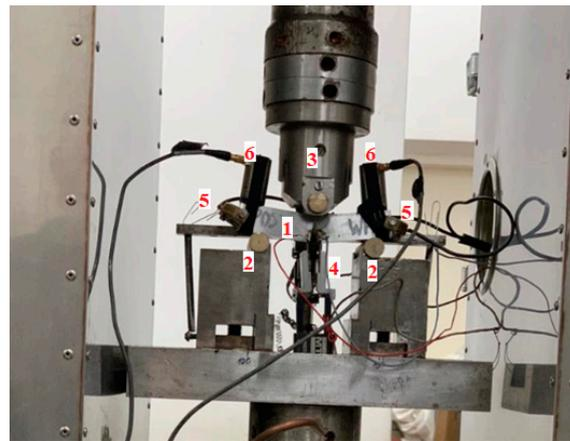
**Figure 1.** The view of the SENB specimen with AE sensors (Zwick-100, ZwickRoel Ulm, Germany) during test: 1—a sample, 2—support, 3—load cylinder, 4—COD extensometer, 5—AE sensors—100–1200 kHz, 6—AE sensors—30–80 kHz.
