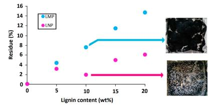
Figure 12. Effect of lignin size and content on the amount of char residue formed during cone calorimeter test.
