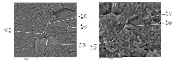
$\textbf{Figure 17.} \ \textbf{SEM} \ \textbf{observations and} \ \textbf{EDX} \ \textbf{analysis} \ \textbf{of} \ \textbf{PLA} \ \textbf{containing} \ \textbf{10} \ \textbf{wt\%} \ \textbf{LNP-SiP.}$
