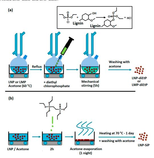
Figure 1. Schematic representation of lignin modification route used for grafting di-EtP (a) and SiP (b).
