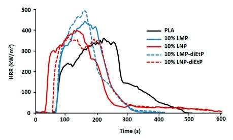
Figure 15. HRR curves of PLA during cone calorimeter test.
