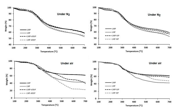
Figure 6. TGA curves of untreated and phosphorylated lignin particles (under air and nitrogen, 10 °C/min).
