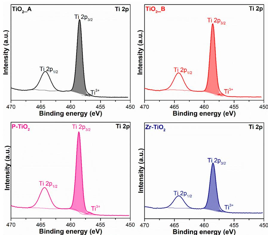
Figure 7. X-ray photoelectron spectra of the samples in the Ti 2p core level.
