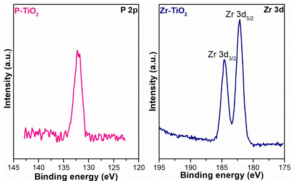
Figure 9. X-ray photoelectron spectra of P 2*p* and Zr 3*d* of P-TiO<sub>2</sub> and Zr-TiO<sub>2</sub>, respectively.
