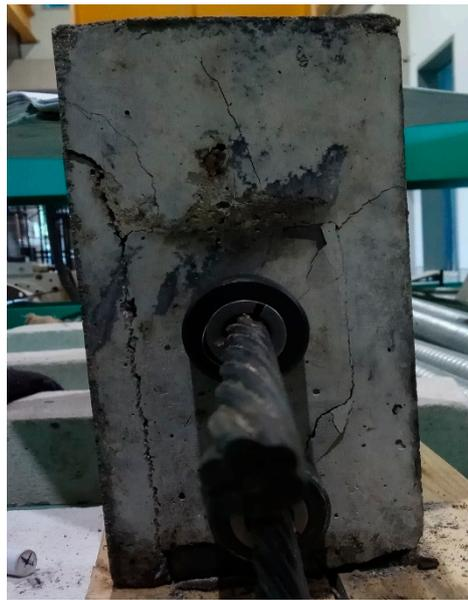
**Figure 7.** Cracks formation at transfer in fly ash based control beam, PSCFY-1.
