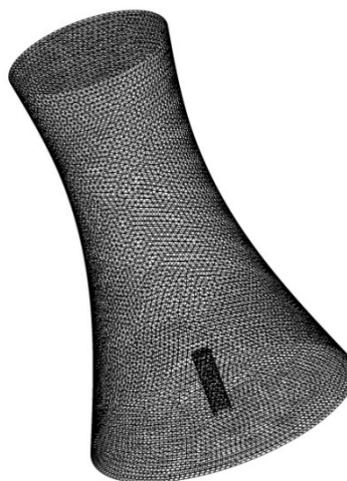
Figure 8. Finite element model of the cooling tower with a flue gas tube.
