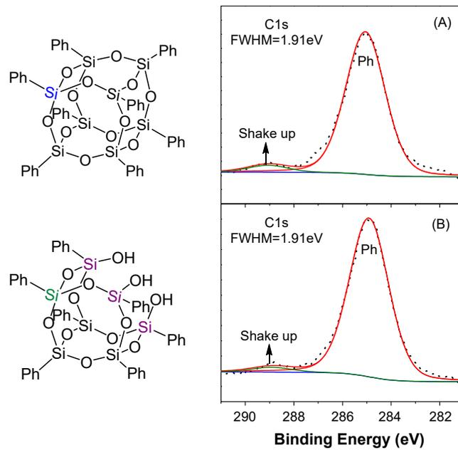
**Figure S5.** XPS C1s of (A) OPS and (B) T<sub>7</sub>-POSS.
