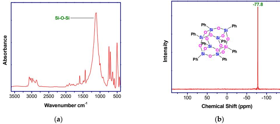
Figure S1. (a) FTIR spectrum and (b) <sup>29</sup>Si NMR spectrum of Octaphenylsilsesquioxanes.
