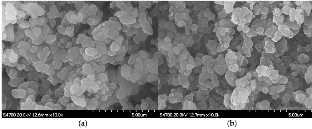
**Figure S4.** SEM morphology of OPS based porous materials with different reaction time (a) 5 h and (b) 20 h.
