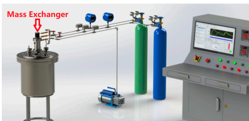
Figure 4. The experiment bench of the oxygen control system.
