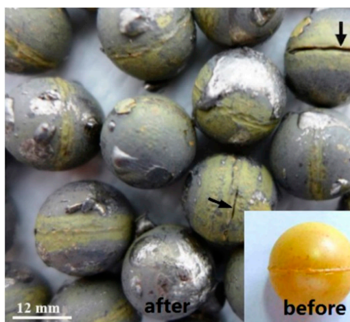
Figure 1. PbO ceramic pellets tested in the CRAFT loop and MEXICO loop [5].
