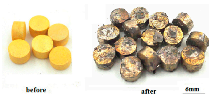
Figure 5. The 3 wt.% Bi 2 O 3 -97 wt.% PbO pellets before and after the flushing experiment.
