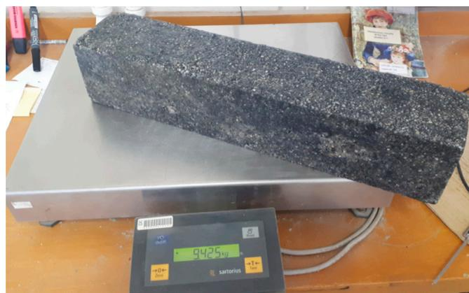
**Figure 6.** Weighing the test sample.
