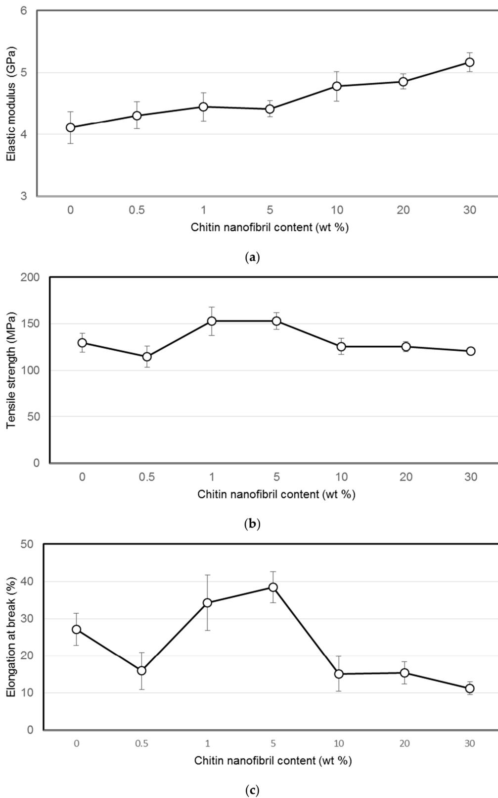
**Figure 1.** (a) Elastic modulus, (b) tensile strength, and (c) elongation at break of pure chitosan and chitin nanofibril-reinforced chitosan films as a function of chitin nanofibril content.
