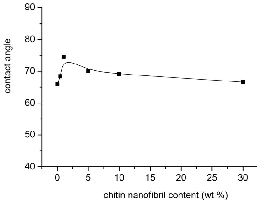
**Figure 3.** Dependence of the water contact angle on the chitin nanofibrils content of chitosan-based composite films.
