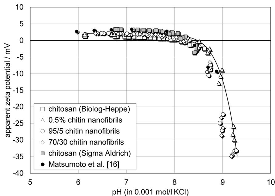
**Figure 4.** pH dependence of zeta potential for chitin–chitosan nanocomposite films. Comparison with pure chitosan films made of chitosan from different suppliers and with electrospun chitosan nanofiber nonwoven [16].
