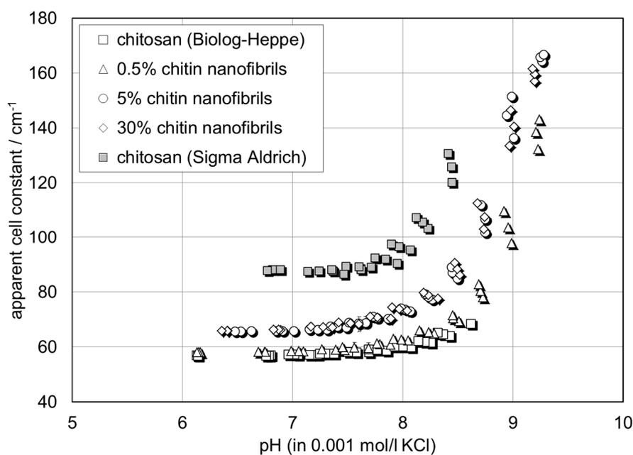
**Figure 5.** pH dependence of apparent cell constant (Equation (2)) of the rectangular capillary channel for chitin–chitosan nanocomposite films. Comparison with pure chitosan films made of chitosan from different suppliers.
