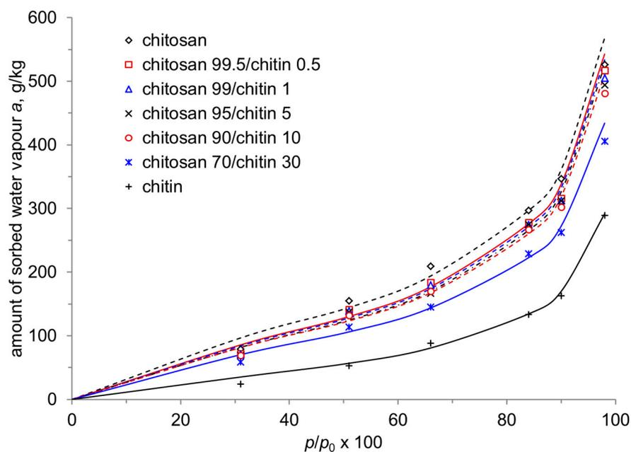
**Figure 2.** The sorption isotherms of water vapour by chitosan–chitin composite films. The symbols represent experimental data and the lines represent the sorption isotherms calculated by Equation (3).
