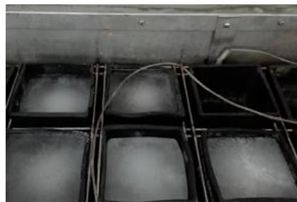
Figure 4. Specimens placed in the rubber sleeves.
