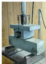
Figure 5. The flexural strength test setup.
