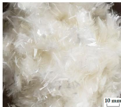
**Figure 2.** The PVA fibers used in this investigation.
