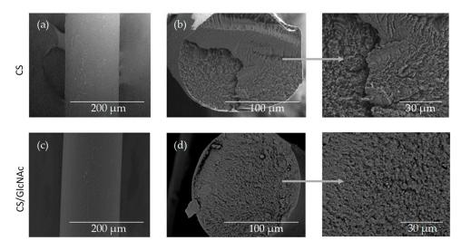
**Figure 3.** SEM micrographs of the surface (**a**,**c**) and the cross-section (**b**,**d**) morphology of the CS and CS/GlcNAc wet-spun filaments.
