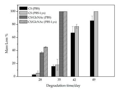
Figure 5. Mass loss of CS and CS/GlcNAc filaments as a function of the degradation time.
