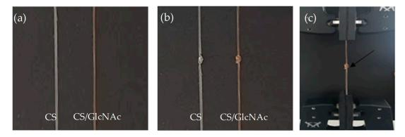
**Figure 2.** Filaments of CS and CS/GlcNAc: non-knotted (**a**); knotted; (**b**) and placed in the Instron machine with the knot approximately midway between the clamps (**c**).
