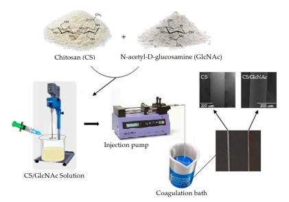
**Figure 1.** Schematic representation of the fabrication of chitosan (CS) and N-acetyl-D-Glucosamine (GlcNAc)-loaded CS wet-spun filaments.
