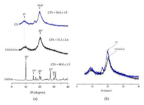
**Figure 4.** XRD patterns of (**a**) the GlcNAc, CS, and CS/GlcNAc wet-spun filaments, and **a** (**b**) comparison of the intensity values.
