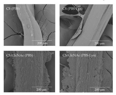
**Figure 6.** SEM images of the CS and CS/GlcNAc filaments after incubation in a phosphate buffered saline (PBS) solution and PBS–lysozyme (PBS–Lyz) at 37 °C for 49 and 35 days, respectively.
