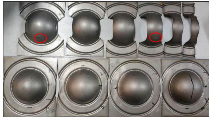
Figure 10. Hemispherical punch stretching tests for part of specimens.
