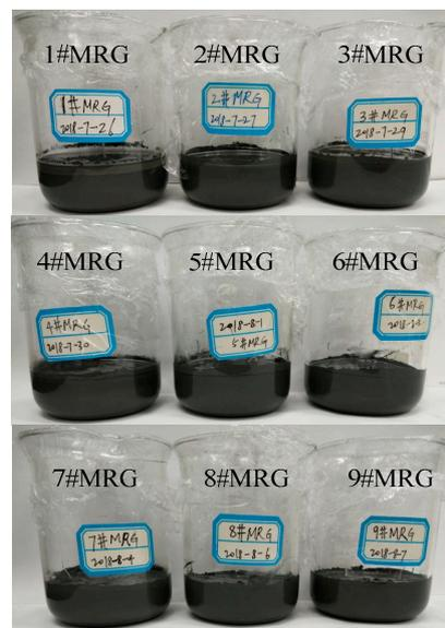
**Figure 2.** Appearance of MR greases after holding in a static state for 30 days.
