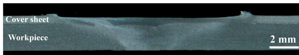
Figure 3. Cross section of the CFSW joint.
