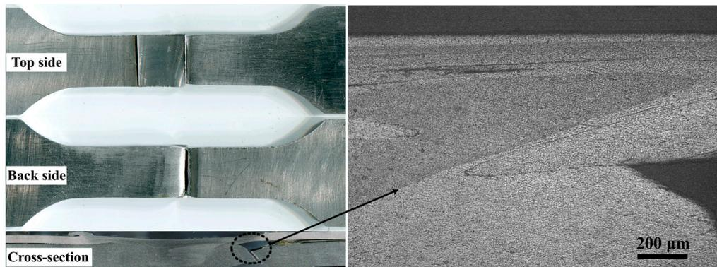
Figure 7. Morphology of the fracture of joints.
