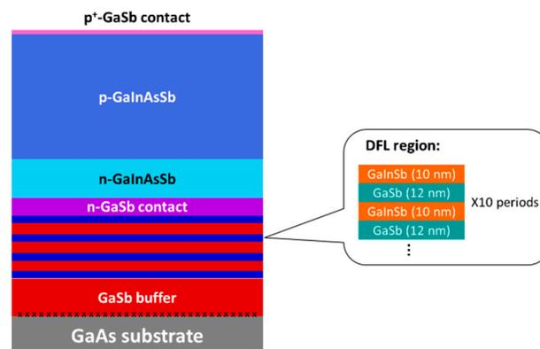
**Figure 1.** Schematic illustration of the GaInAsSb P-N diode grown on GaAs substrate with interfacial misfit (IMF) arrays and four dislocation filtering layer (DFL) regions. The details of the DFL regions are included in the inset.
