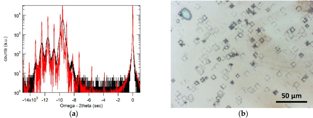
**Figure 4.** (a) measured (black curve) and simulated (red curve) XRD spectra of the GaInSb/GaSb DFL regions; (b) optical microscopy image of the sample after EPD measurements.
