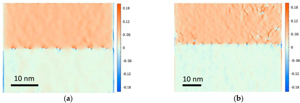
**Figure 3.** Geometric phase analysis (GPA) images of the GaSb/GaAs interface: (a) without TDs; (b) with TDs.
