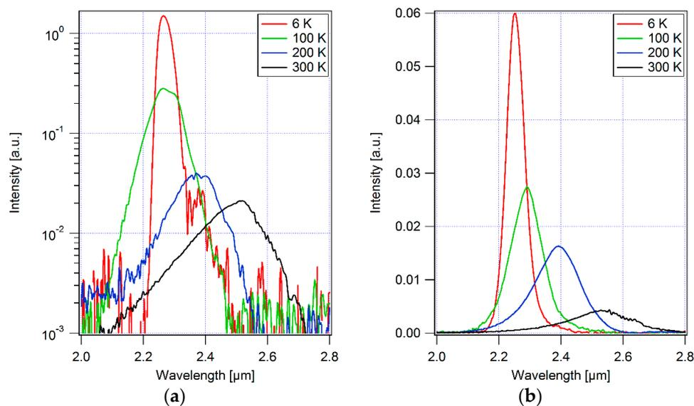
**Figure 5.** (a) Photo-luminescence spectra of the GaInAsSb material grown on GaAs at different temperatures; (b) electro-luminescence spectra of the GaInAsSb P-N diode grown on GaAs at different temperatures.
