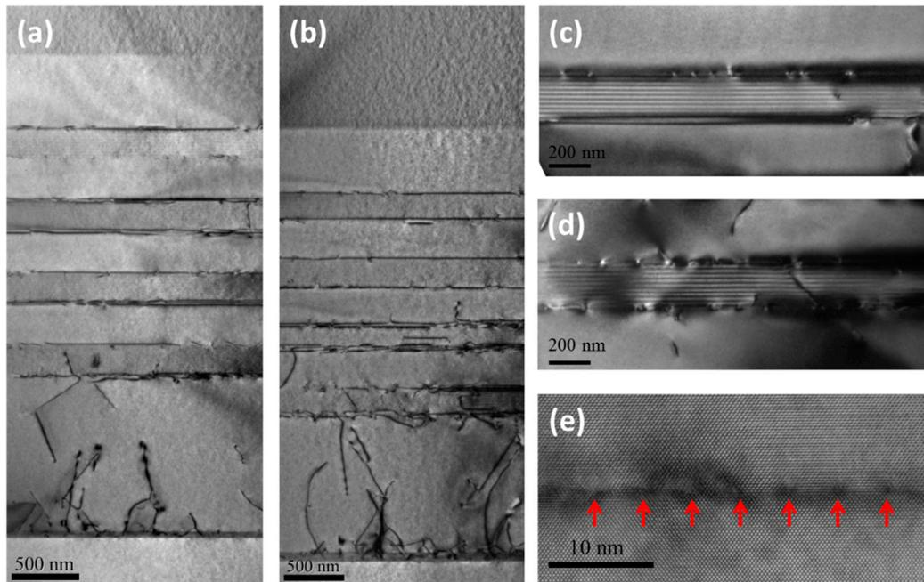
**Figure 2.** Cross-sectional TEM images of the metamorphic buffer region (a) with low TD density, and (b) with high TD density. High-resolution TEM images revealed the details of (c) the top DFL region, (d) the bottom DFL region and (e) the GaSb/GaAs interface.
