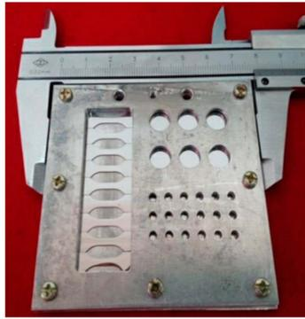
**Figure 2.** Clamping fixture holding the specimens during proton irradiation.
