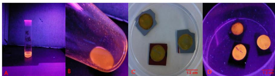
**Figure 2.** (A)  $^{11}\text{C}_{11}$  alkyl-capped SiQDs as a toluene sol and (B) after evaporation of the toluene; both photographs taken under illumination with an Hg lamp ( $\lambda = 365 \text{ nm}$ ) to show the orange fluorescence. (C) The porous silicon, an approximately circular, brown–yellow area formed on the top of the silicon chip. (D) A fluorescent image of porous silicon under UV-lamp (Hg,  $\lambda = 365 \text{ nm}$ ).
