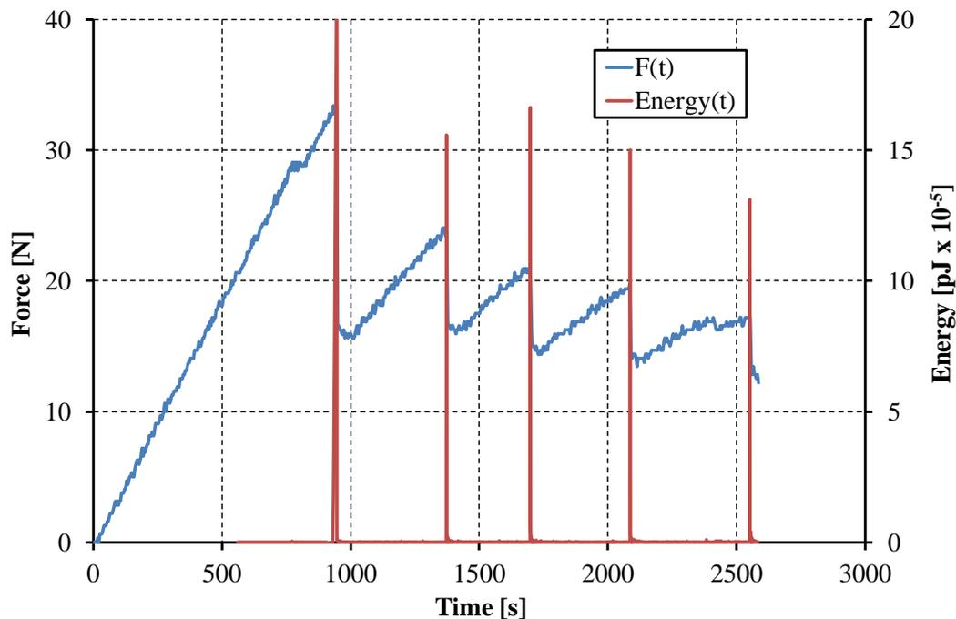
Figure 4. Example of detecting the peak load using the energy of AE.
