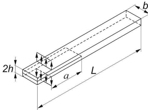
Figure 1. Double cantilever beam (DCB) specimen configuration.
