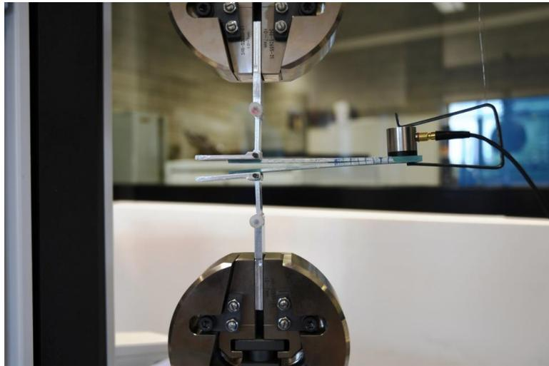
**Figure 2.** Loaded DCB specimen with AE sensor.
