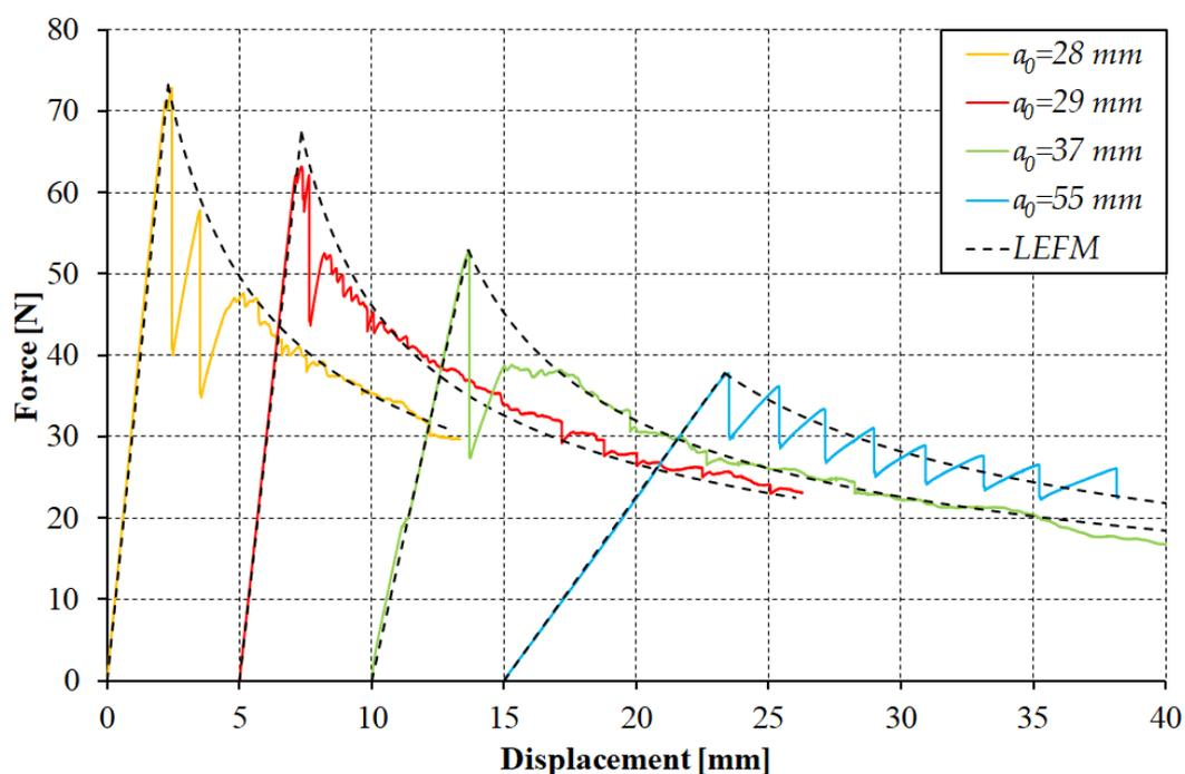
Figure 3. Load-displacement curve obtained from the DCB tests.
