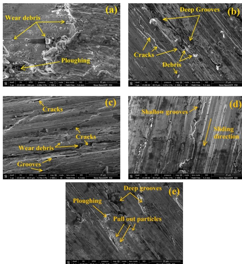
**Figure 10.** Representative micrographs of selected composite after wear test under 15-N normal load, 4.69 m/s sliding velocity and 1500 m sliding distance of (a) A-1, 0 wt.% MD; (b) A-2, 1.5 wt.% MD; (c) A-3, 3 wt.% MD; (d) A-4, 4.5 wt.% MD; (e) A-5, 6 wt.% MD reinforced composites.
