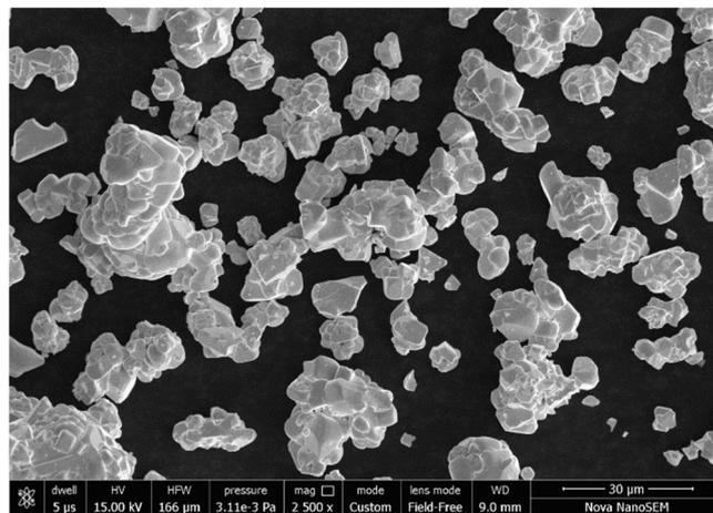
**Figure 1.** Scanning electron microscope (SEM) micrograph of marble dust powder.
