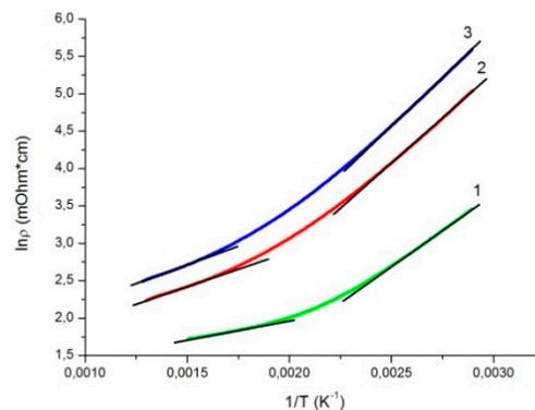
**Figure 5.** Reciprocal temperature dependence of the  $\text{Gd}_{0.2}\text{Sr}_{0.8}\text{FeO}_{3-\delta}$  logarithmic resistivity. Black straight lines show the thermal activation law processing: (1) first heating, (2) first cooling, and (3) third cooling.
