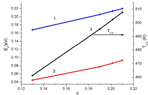
**Figure 6.** Dependencies of the activation energy  $E_a$ : (1) is the temperature region below the electronic transition and (2) is the high-temperature region, and (3) semiconductor–semiconductor transition temperature  $T_{p-p}$  on the oxygen nonstoichiometry index.
