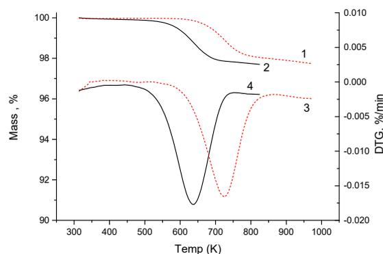
**Figure 2.** (1, 2) TG and (3, 4) DTG curves of temperature-programmed reduction of the  $\text{Gd}_{0.2}\text{Sr}_{0.8}\text{FeO}_{2.87}$  compound in the 5%  $\text{H}_2$ -Ar mixture flow at heating rates of 2 (black solid curve) and 20 K/min (red dotted curve).
