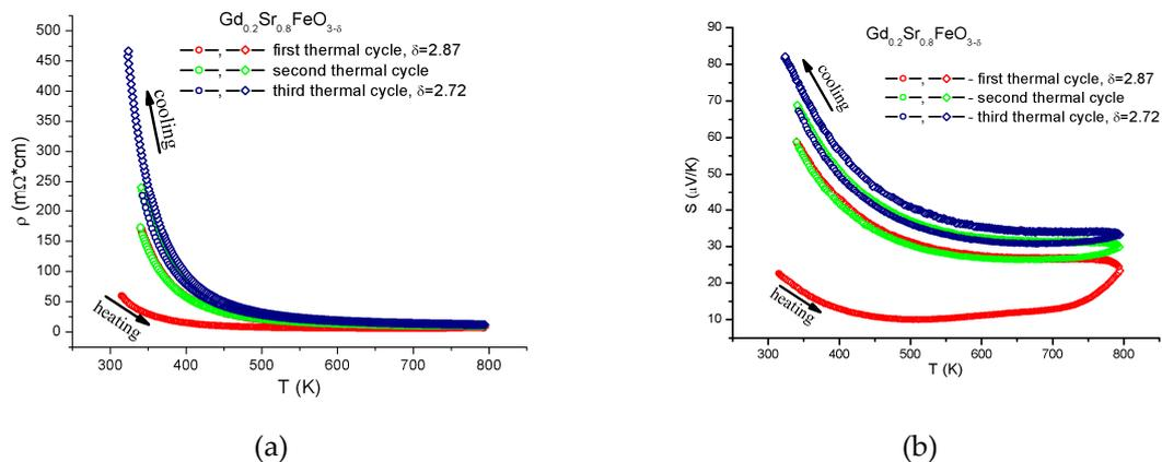
**Figure 3.** Temperature dependences of (a) the resistivity and (b) thermopower for three continuous heating-cooling cycles.
