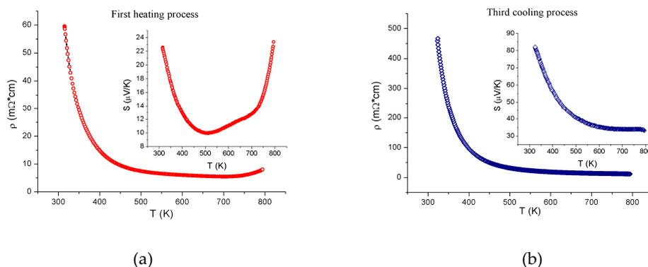
**Figure 4.** Temperature dependences of the resistivity and thermopower (insets) during (a) the first heating and (b) the third cooling.
