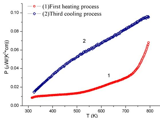
**Figure 7.** Temperature dependencies of the power factor  $P$  for the first heating ( $\delta = 0.13$  at  $T = 300$  K) (1) and the third cooling ( $\delta = 0.21$ ) (2).
