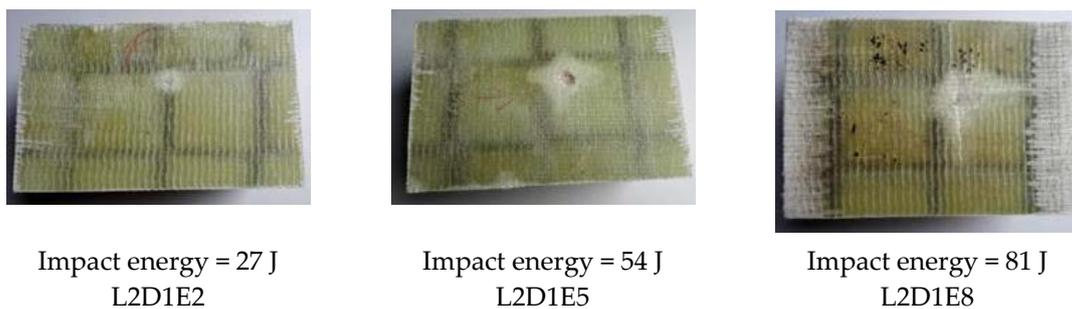
**Figure 9.** Impact damage at Location L2.
