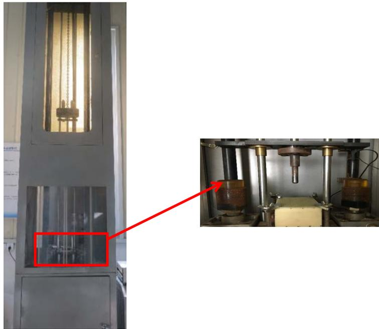
**Figure 3.** The drop tower apparatus.
