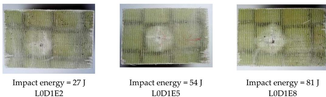
**Figure 7.** Impact damage at Location L0.
