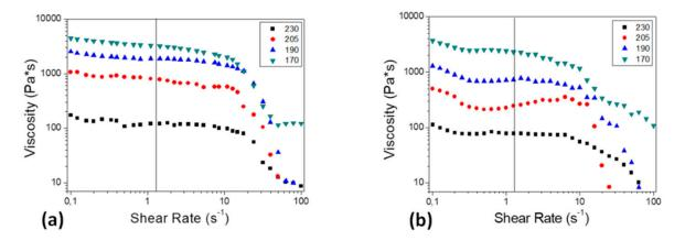
**Figure 5.** Viscosity vs. shear rate at different temperatures of interest for (**a**) neat PDMS and (**b**) composite Na–CMC/PDMS filaments.
