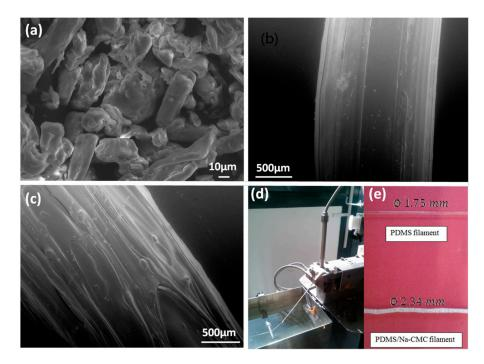
**Figure 3.** Scanning Electron Microscopy (SEM) images of the (**a**) employed Na–CMC powder; (**b**) bare PDMS filament surface; (**c**) Na–CMC/PDMS composite filament; photographs of (**d**) one filament during the extrusion process and (**e**) the two kinds of obtained filaments.
