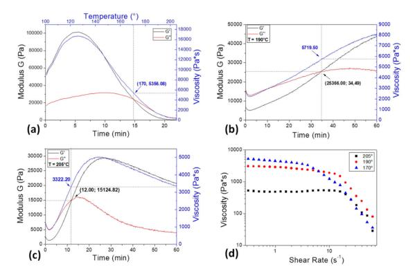
**Figure 2.** Rheological analysis on PDMS pellets: (**a**) dynamic rheological ramp test; (**b**) isothermal characterization at 190 °C and (**c**) at 205 °C; (**d**) viscosity vs. shear rate at different temperatures of interest.
