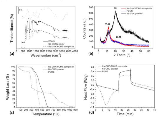
**Figure 1.** Comparison of the properties of neat polydimethylsiloxane (PDMS), sodium carboxymethylcellulose (Na–CMC) powder, and the Na-CMC/PDMS composite, in terms of: (a) Fourier Transform Infrared Spectroscopy (FTIR) spectra; (b) X-ray Diffraction (XRD) patterns; (c) thermogravimetric analysis (TGA) and (d) Differential Scanning Calorimetry (DSC) thermograms.
