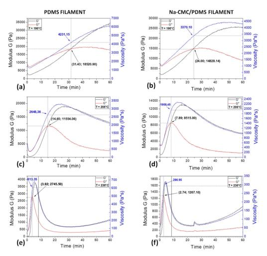
**Figure 4.** G', G" and viscosity curves as a function of time under varying process temperature, for both the (**a**,**c**,**e**) bare PDMS and (**b**,**d**,**f**) composite Na–CMC/PDMS filament.
