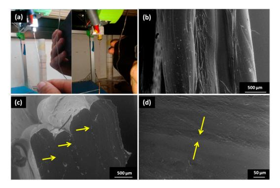
**Figure 6.** Photos of (**a**) the neat PDMS and composite Na–CMC/PDMS filaments used in FDM; SEM images, at different magnification, of (**b**–**d**) the composite filament printed in layers. Arrows indicate the interface between different layers.
