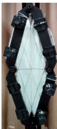
Figure 13. LT-t in the deformed position sample (1.05 rad shearing angle).
