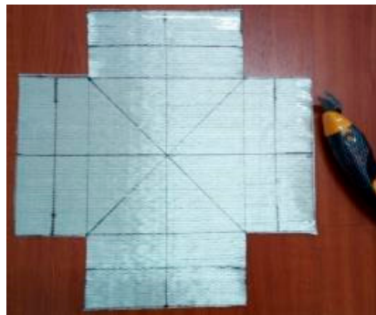
Figure 8. A sample of UD-t after cutting by “e-scissor” with the marking lines.
