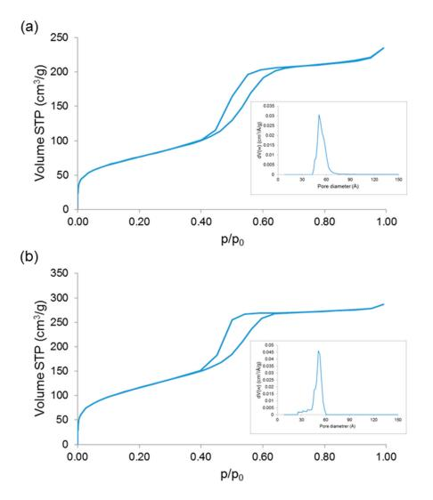
**Figure 8.** Nitrogen adsorption-desorption isotherms of (**a**) 1Cu-MBG and (**b**) 5Cu-MBG. Insets in both pictures report the pore size distribution.
