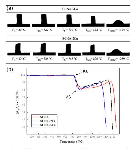
**Figure 1.** Results of HSM: (**a**) silhouettes of the Cu-doped SCNA-based glasses sample at different characteristic temperatures upon heating ( $T_R$  room temperature,  $T_{FS}$  first shrinkage,  $T_S$  softening,  $T_{MS}$  maximum shrinkage,  $T_{FLOW}$  flowing); (**b**) shrinkage variation as a function of temperature ( $A_0$  area of the silhouette at room temperature,  $A_T$  sample area at the current temperature).
