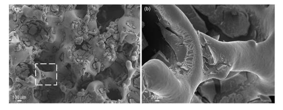
**Figure 9.** SEM micrographs of (**a**) the porous structure of 5Cu-MBG-SCNA scaffold (magnification  $100 \times$ ) and (**b**) detail of a trabecula (dashed square in (**a**)) coated by the MBG layer (magnification  $500 \times$ ).
