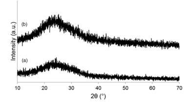
Figure 6. Wide-angle XRD pattern of (a) 1Cu-MBG and (b) 5Cu-MBG.
