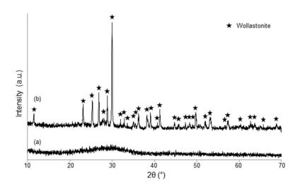
**Figure 2.** Wide-angle XRD pattern of (**a**) as-quenched SCNA-2Cu and (**b**) SCNA-2Cu thermally treated at 1000  $^{\circ}$ C for 3 h.
