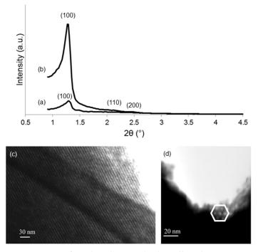
**Figure 7.** Mesoporous structures of Cu-doped MBGs: (top) small-angle XRD pattern of (**a**) 1Cu-MBG and (**b**) 5Cu-MBG; (bottom) STEM images of 5Cu-MBG recorded along (**c**) [100] and (**d**) [001] directions. In (**d**) the typical hexagonal symmetry of the mesopores is emphasized.
