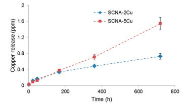
Figure 5. Profiles of copper release from SCNA-2Cu and SCNA-5Cu scaffolds following immersion in SBF.
