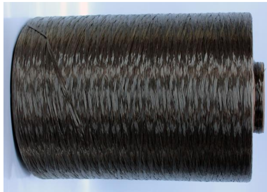
Figure 1. Continuous untwisted basalt fibers.
